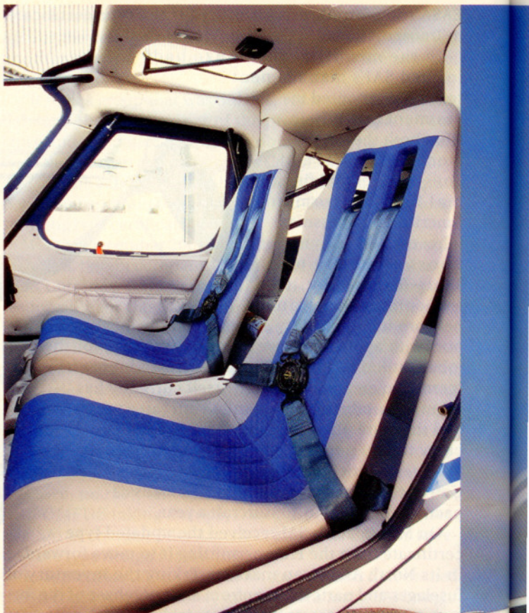
A four-point harness and rugged seats are just two of the many safety features found in the 160. The addition of a BRS airframe parachute will up the safety ante further still.
